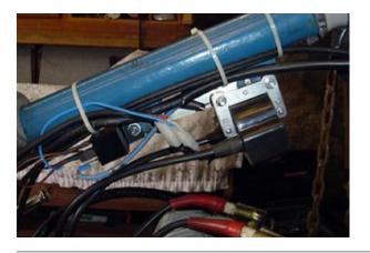
Screw the new HT-cable into the ignition coil and fasten the coil at the place of the original one. Use the provided fixing plate. Leave one of the screws loose, you have to fasten a ground cable from the ignition coil harness here.
