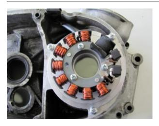
Put the preassembled stator unit onto the engine housing. Fasten it down with the 3 provided screws.
