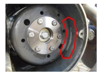
When you put back the engine housing onto the engine you'll see that the rotor scratches at it (see picture left).
