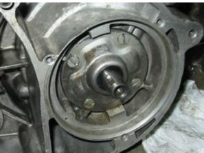
Disconnect all cables from your old generator, regulator and the ignition coil and remove those parts.
