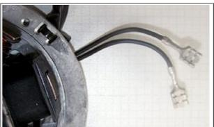
The 2 black wires running from the stator coil carry the voltage for lights, horn, flashers etc. They have nothing to do with ignition.
