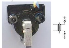
In our twin outlet coils both ends of the secondary go to the spark plugs.
