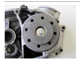
In that position fasten the rotor down with the provided M7x50 screw and washer.
