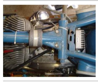
Fasten the rectifier/regulator and (if you use the relay option) the relay at a conveniend place.
